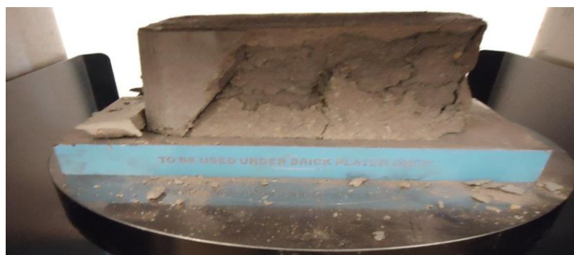
Fig. 4: Failure pattern of SCEB showing a shear of shell and core [13]
