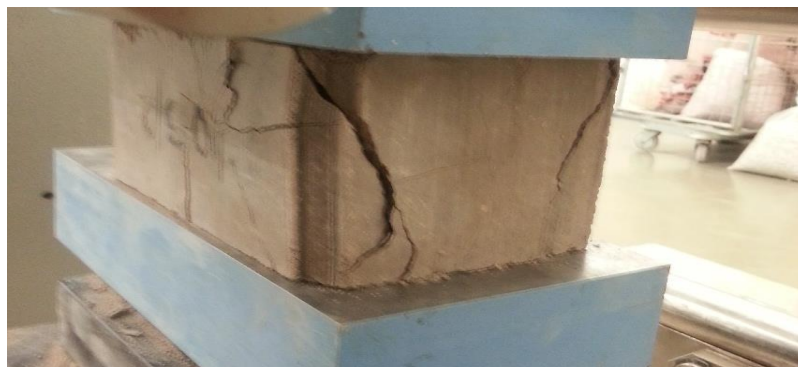
Fig. 3 Cracks on shell at failure
